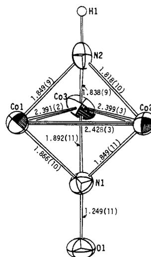
**Figure 4.** The bicapped tricobalt  $\text{Co}_3(\text{NO})(\text{NH})$  core of the  $[\text{Co}_3(\eta^5\text{-C}_5\text{H}_4\text{Me})_3(\mu_3\text{-NO})(\mu_3\text{-NH})]^+$  monocation (IIIb) with its independent interatomic distances under crystallographic  $C_1$ -1 site symmetry. The position of the nitrene hydrogen atom was located from an electron-density difference synthesis.
